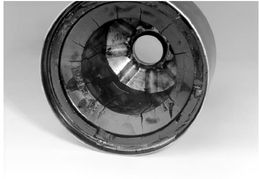
Figure 15 - Centrifuge Rotor Cover from Engine 2 (Second Oil Drain - 700-1400 Hours)
