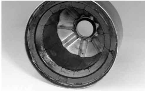
Figure 14. Centrifuge Rotor Cover from Engine 2 (First Oil Drain - 0-700 Hours)
