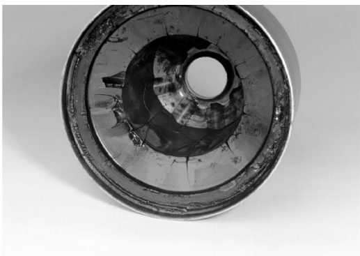
Figure 16 - Centrifuge Rotor Cover from Engine 2 (Third Oil Drain - 1400-2100 Hours)
